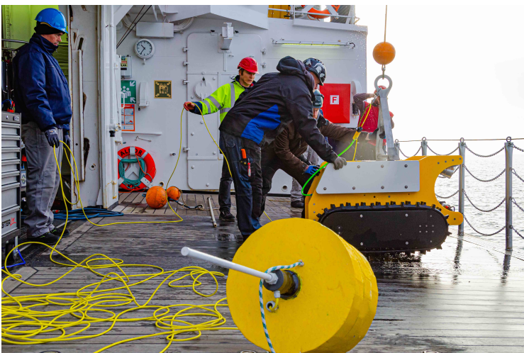
Fig. 6. Crawler control via surface float for deployments in coastal areas from ships. The crawler can be deployed from a vessel of opportunity. Test cruise in November 2019. The WLAN connection can be extended to several kilometers in water depth down to 200 m.
