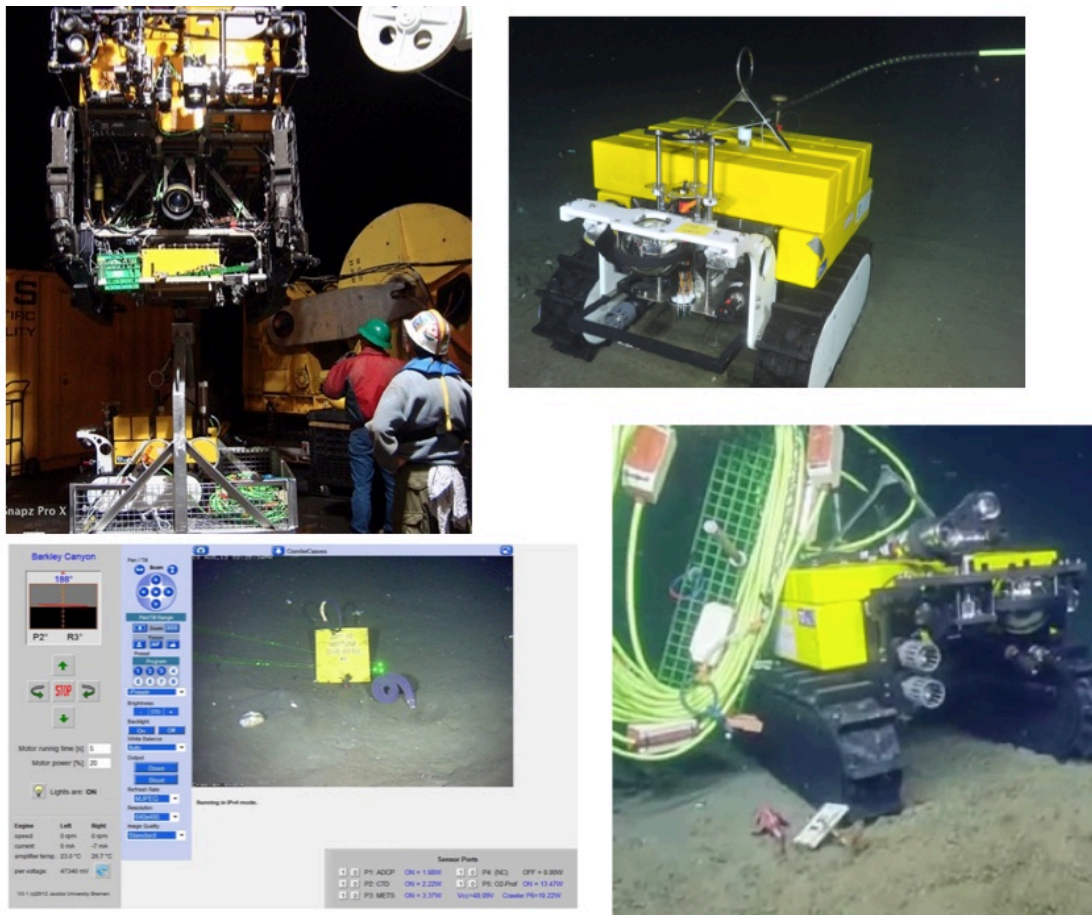
Fig. 3 Crawler technology, operational at the Ocean Networks Canada cabled observatory since 2010 for 12 – 18 months deployments at 900 m water depths in Barkley Canyon
