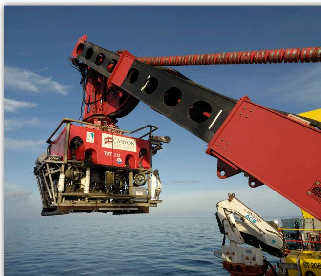
*A remotely operated vehicle (ROV) being deployed to study the seafloor. © Nautilus Minerals*
