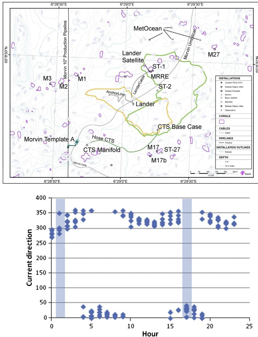
**Fig. 6.** Two examples of the distribution of the mud cloud as visually mapped by ROV on November 30, 2009 at 01:25 AM (orange line) and 17:30 PM (green line) (upper panel with courtesy R. Welzin, Statoil). Lower panel shows current direction during that day and the difference between the two sampling periods (indicated in hatched columns).
