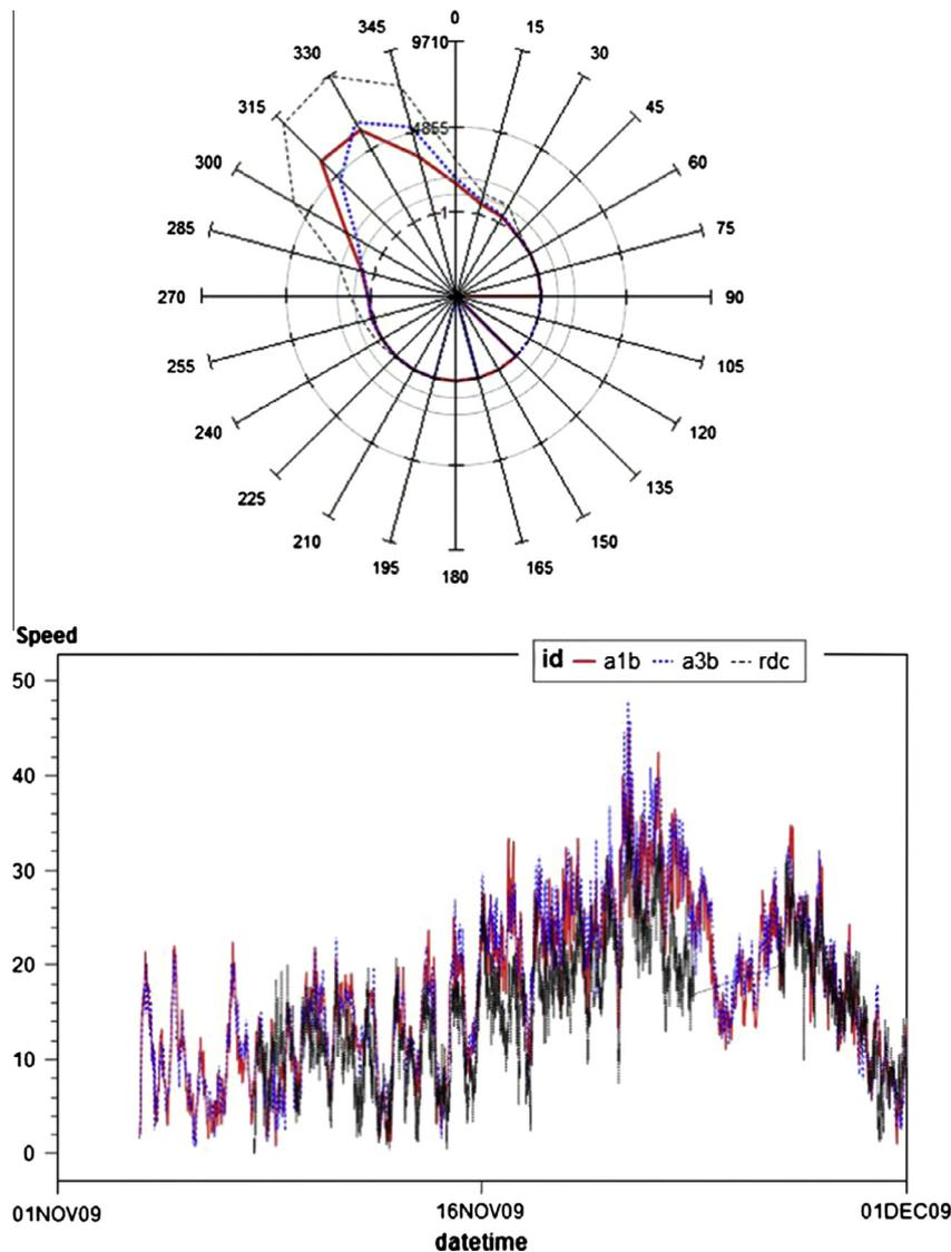
**Fig. 5.** Current speed ( $\text{cm}^{-1}$ ) and direction as observed by the RDCP and the two of the moored Aquadopp point measurements. Upper panel shows prevailing direction of speed recorded as number of observation in various directions. ID identifies the moorings (a1b and a3b compared to the RDCP (rdc)). Lower panel shows the current speed variation of the same instruments (break in time series of the RDCP is due to maintenance).
