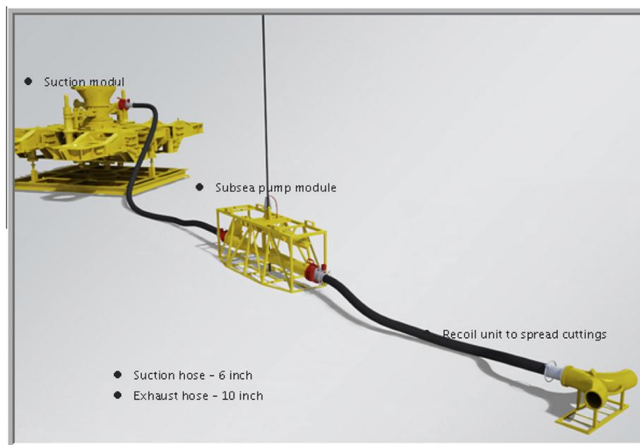
Fig. 2. Illustration of the transportation system of the cuttings to a location away from the drilling site.
