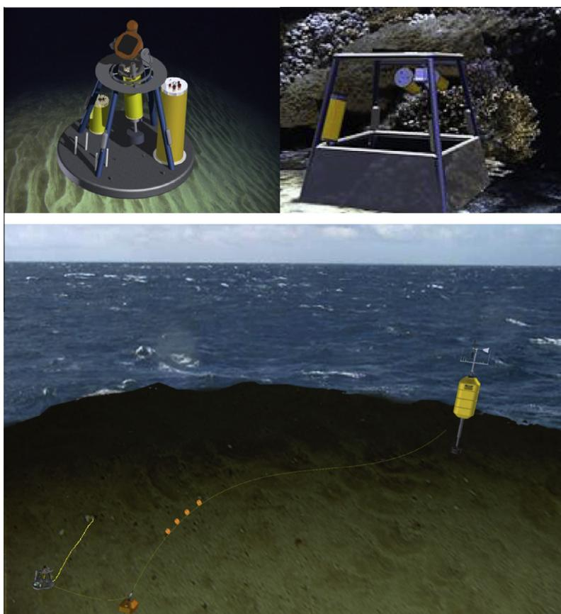
Fig. 3. The design of the sensor platform with satellite camera and a surface communication buoy.
