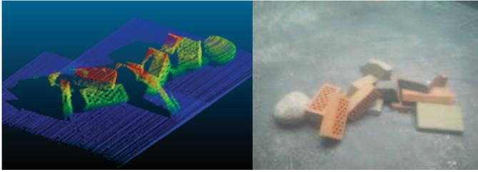
Figure 2 3D reconstruction (left) of an underwater obstacle scene (right) using a line structured light method with a visible laser light.
