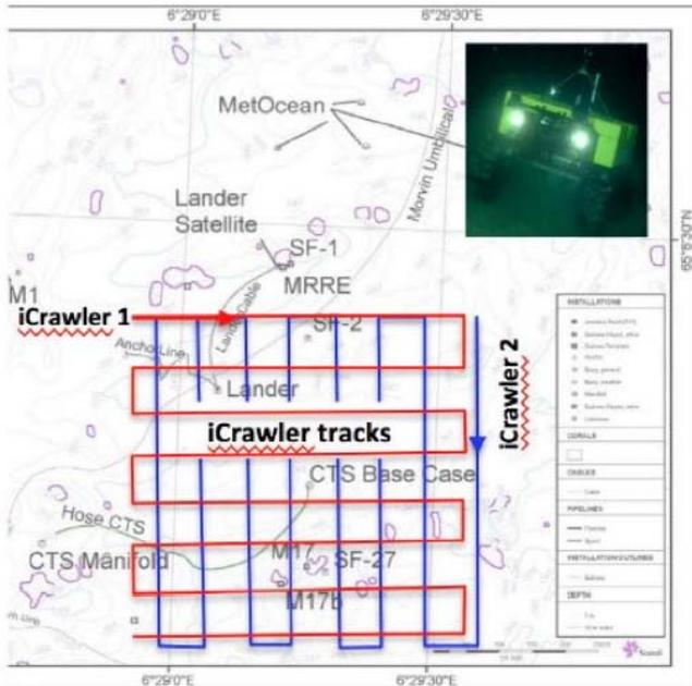
Figure 5 Typical mission for iCrawlers at an exploration site
