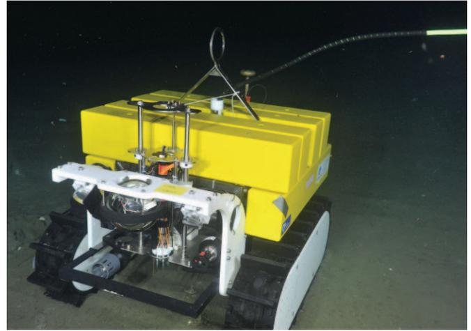
Figure 3 Teleoperated crawler during a transect to a gas-hydrate mound. A range of components are indicated, including the Max Planck sediment profiler
