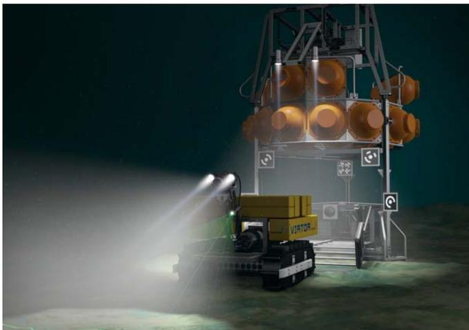
Figure 7 Sketch of the complete system for the proposed 2017 ROBEX demo-mission to Svalbard with RV Polarstern (source: GEOMAR)
