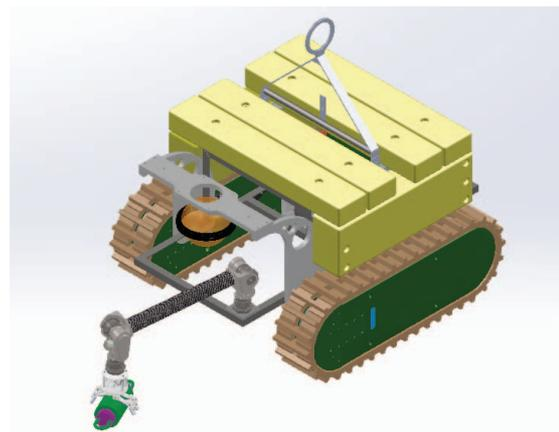
Figure 4 iCrawler with camera guided gripper for the relocation of sensors
